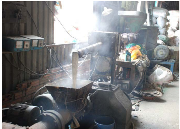
Melting process in a plastic recovery factory on Ao Doi street
