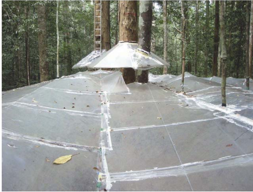
Fig. 4 Big umbrella set for the experiment to artificially cause drought for a target tree.
