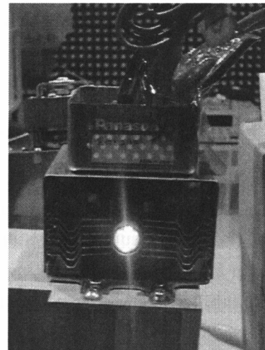
Figure 2.11: Photo of the magnetron for the measurements of the filament temperature. The light of the filament is seen through a crystal plate.
