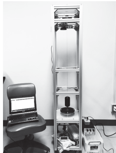
Fig. 6. Photograph of the portable and free-standing pendulum device
