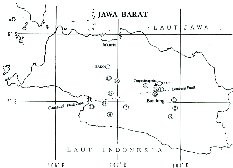
Fig. 1 GPS network in west Jawa. CIAT and BAKO are GPS stations at Ciatiri and BAKOSURTANAL in Cibinong, respectively. 1: Nagreg, 2: Leles, 3: Garut, 4: Cikalongwetan (TTG, 95), 5: Lembang, 6: Cibodas, 7: Sukanegara, 8: Sagaranten, 9: Bojonglopang, 10: Kiaradua (LIPI), 11: Pelabuhanratu, 12: Cisaat, 13: Ciawi, 14: Tugu, 15: ITB1.
