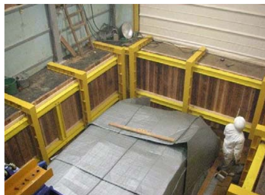
Photo 5 Layout of Earth Retaining Walls
