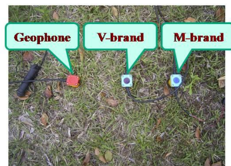
Figure 3. Sensors used for the experiment. Left: conventional geophone. Middle: V-brand MEMS accelerometer. Right: M-brand MEMS accelerometer.
