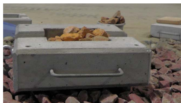
Photo 10 Towing test of Counter weight block
