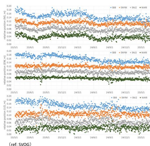
Fig. 5 Comparison between SBB and adjacent GNSS stations
