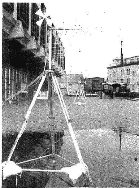
Photo 1 Anemometers set on a tripod.
