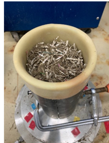
Figure 3.25 Specimen for triaxial test
