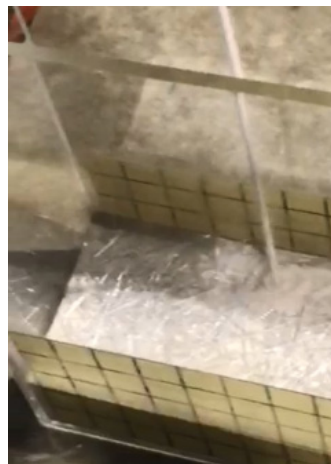
Figure 5.12 Installing fiber-sand mix layer for centrifuge model
