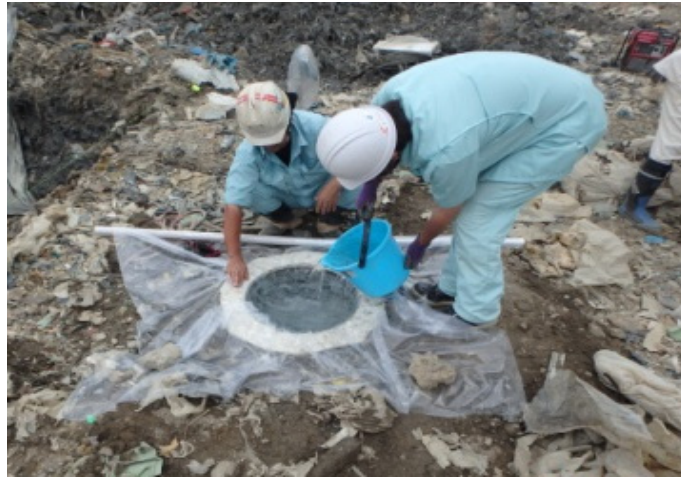
Figure 3.3 In situ wet density test
