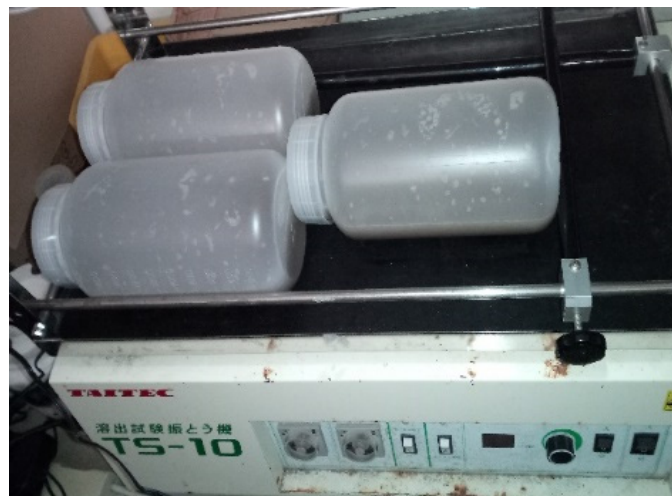
Figure 4.17 Laboratory batch leaching test
