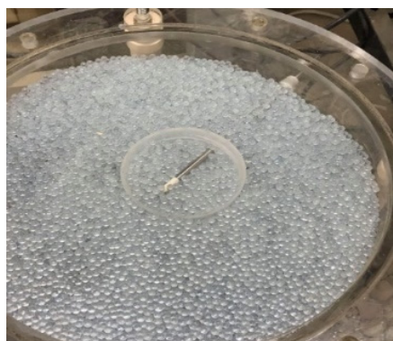
Placing leachate collection tube in column
