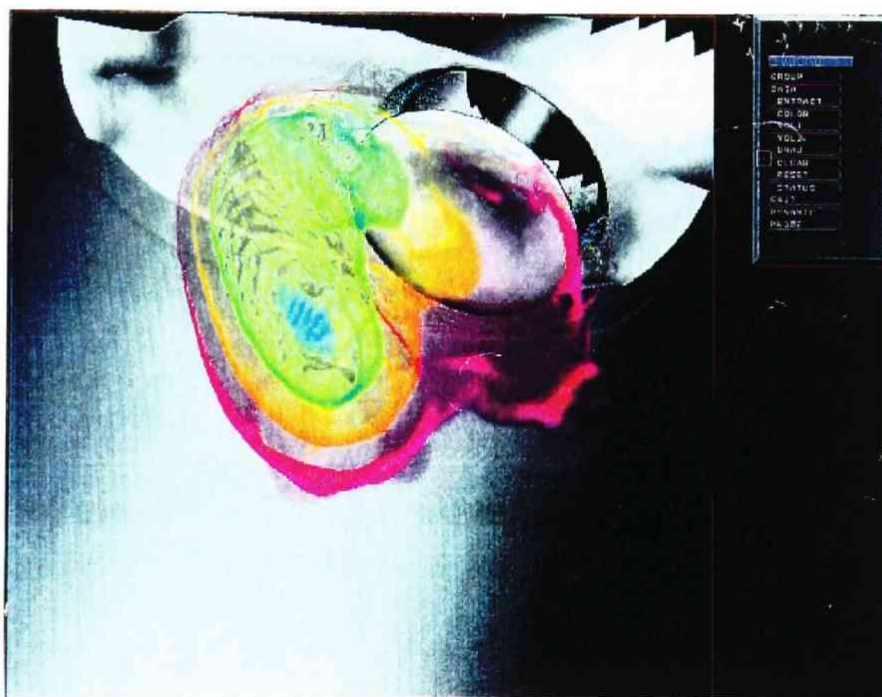
Figure 6.14: Identification of low-pressure region under the valve
