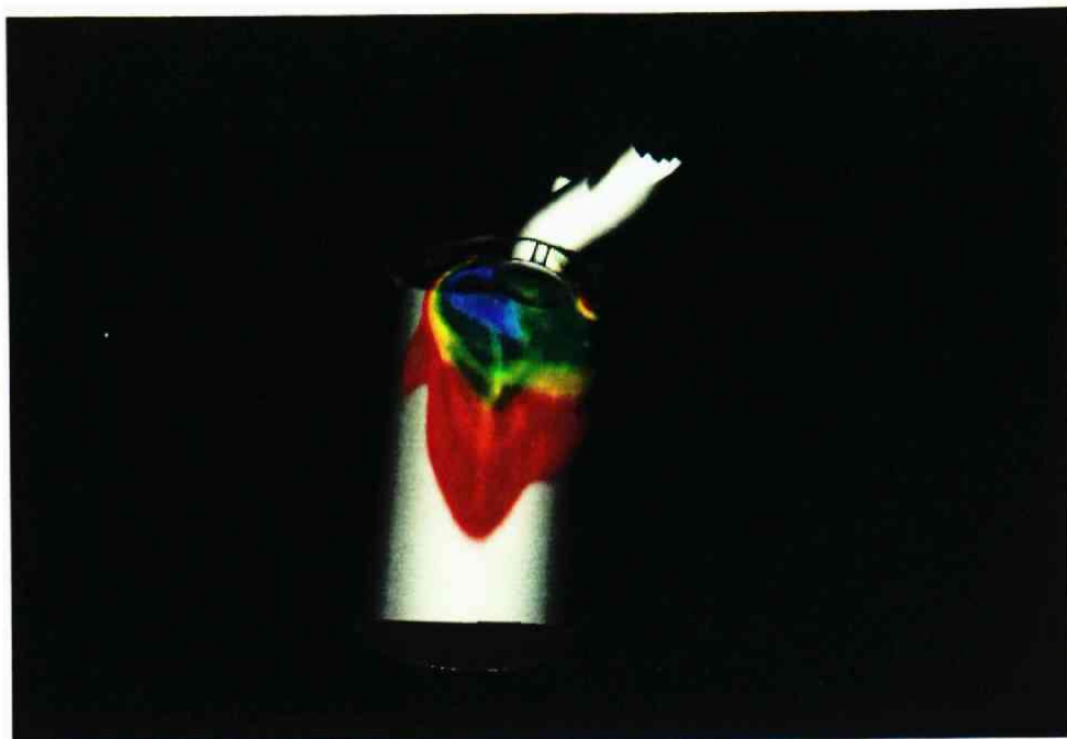
Figure 6.13: Cloudy representation of the calculated pressure fields (372,500 cells)
