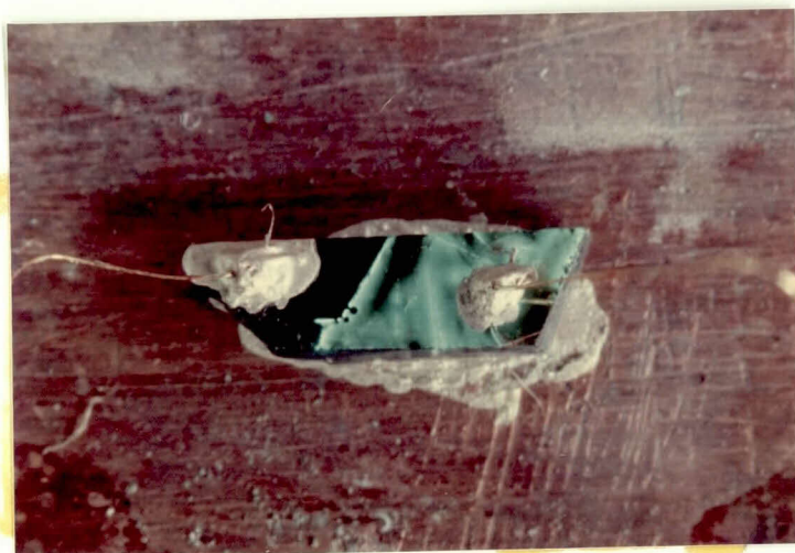
(2) Blue electroluminescence of 6H-SiC diode (300 K) prepared by liquid-phase epitaxial growth (See text p. 80).
