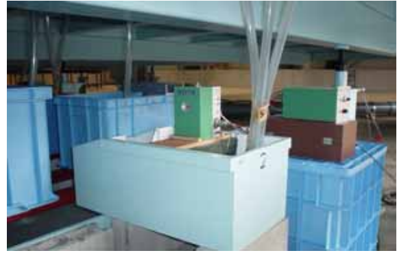
Photo 6 Weirs, level meters, and buckets for discharge measurements. (left : downstream end, right : beneath the model)
