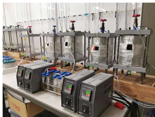
Photo 3.2 On-going hydraulic conductivity test with modified flexible-wall permeameter
