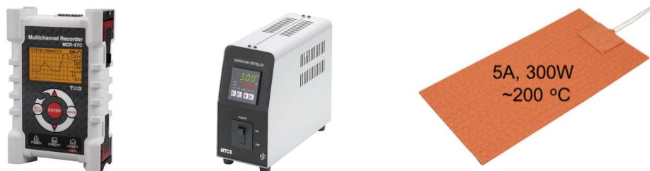
Photo 3.1 Data logger, temperature regulator, and rubber heater used in this study
