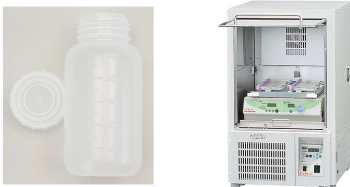
Photo 2.1 Bottle, oscillator, and thermostat for batch test.
