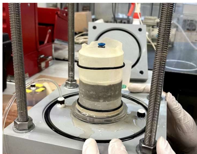
(d) Specimen covered by rubber membrane.
