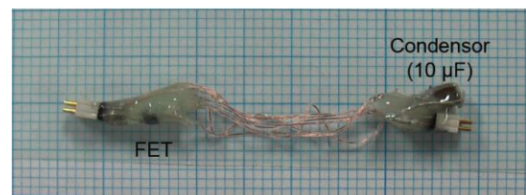
Figure 16 | Impedance matching circuits for neural signal recording. Top: circuits for 1 channel of neural signals. Bottom: photograph of the impedance matching circuits, embedded within the wire bundle between the microdrive and WIF. The 10-pin connector with a FET (left) is connected to the microdrive and that with a condenser (right) is connected to the WIF.
