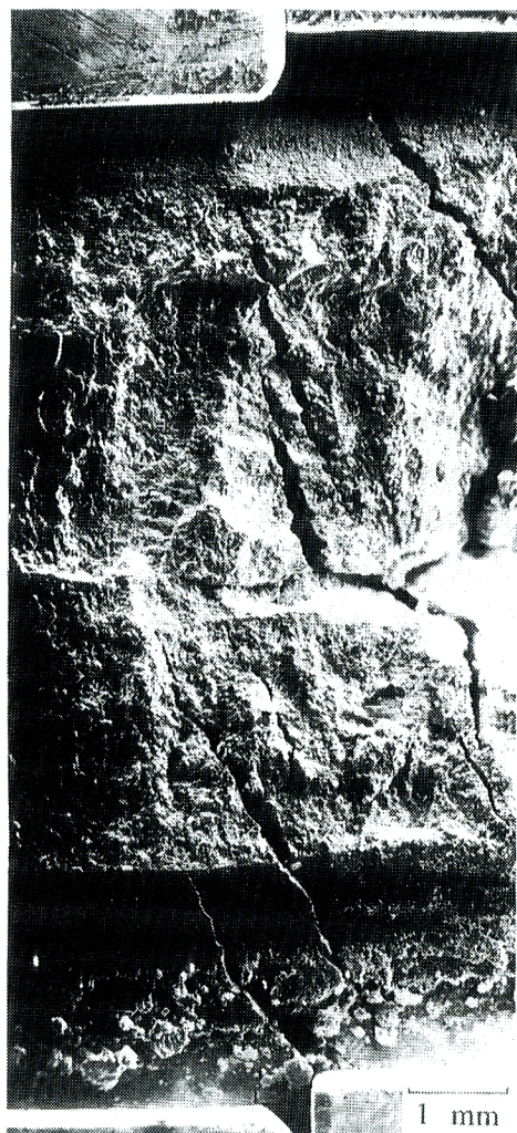
Photo 1. Riedel shear plane (diluvial clay; V-section).
