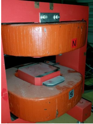
Figure 2.8: Beam dump bending magnet before installation (left) and during installation (right).
