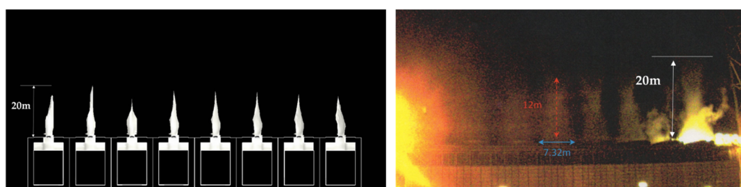
Figure 9. Comparisons of calculated and observed visible plume under dry and wet operation.
