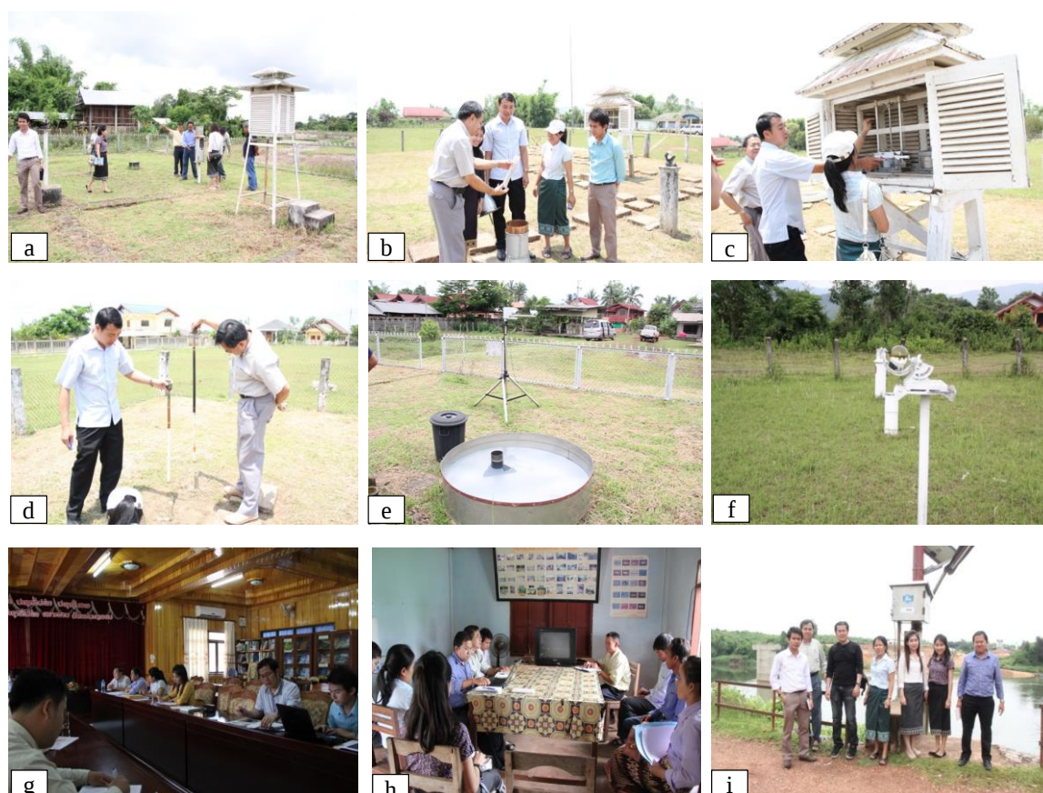
Figure 2.4 Pictures of the meteorological station: (a) station site; (b) rain gauge; (c) temperature measurement; (d) relative humidity; (e) evaporation; (f) sunshine hours; (g) discussion with district staff; (h) discussion with local staff and (i) technical staff team of Natural Resource and Environmental Department in Laos.
