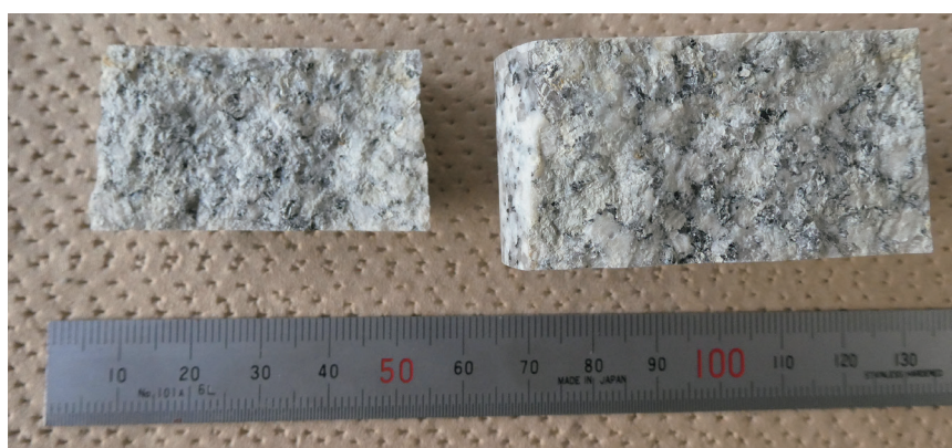
Fig. 13 Photograph of fracture surface of specimen TG-f3 after permeability measurement using water including clays. The upper side in this photo is the upstream side for the permeability measurement.
