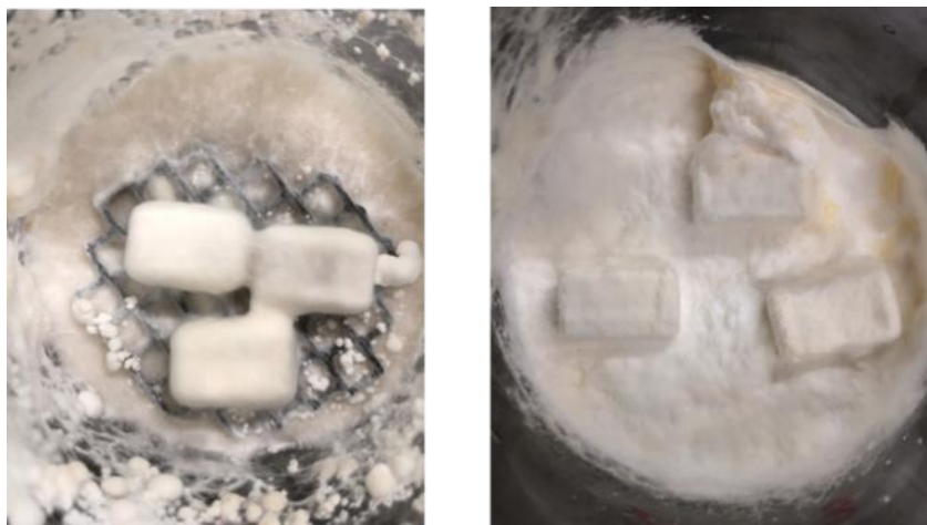
Fig. 4.2 Wood Specimens after 12 weeks exposure of decay tests. Left: Trametes versicolor (COV), Right: Fomitopsis palustris (TYP).
