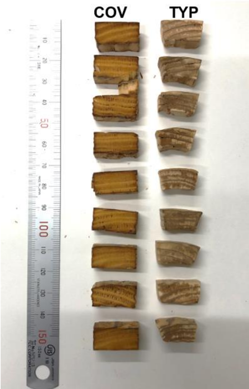
Appendix 4.7 CJ-SW samples after exposure to decay test.
