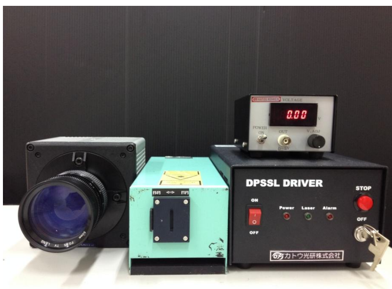
Fig. B.3 Equipments used in flow visualization experiment, showing a high-speed camera, laser generator and its controller.
