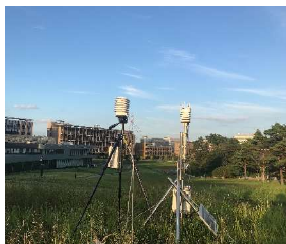
Photo 2 Test observation of air temperature and air humidity sensor with 3D-printed radiation shield. Left side is developed system and right side is WXT536 for validation.
