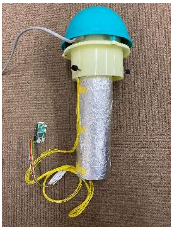
Photo 3 Forced ventilation system
