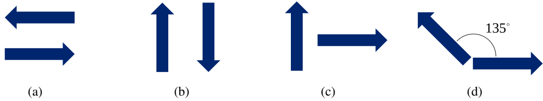
Fig. 4.14 Prescribed directions for the two-dimensional design problem: (a) Prescribed directions along the x -axis; (b) Prescribed directions along the y -axis; (c) Prescribed directions with the angle between them being 90^\circ ; (d) Prescribed directions with the angle between them being 135^\circ .
