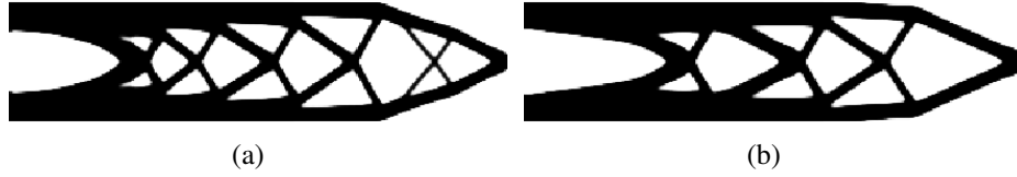
Fig. 5.9 Obtained optimized configurations for (a) l_C = 0.5L ; and (b) l_C = L .
