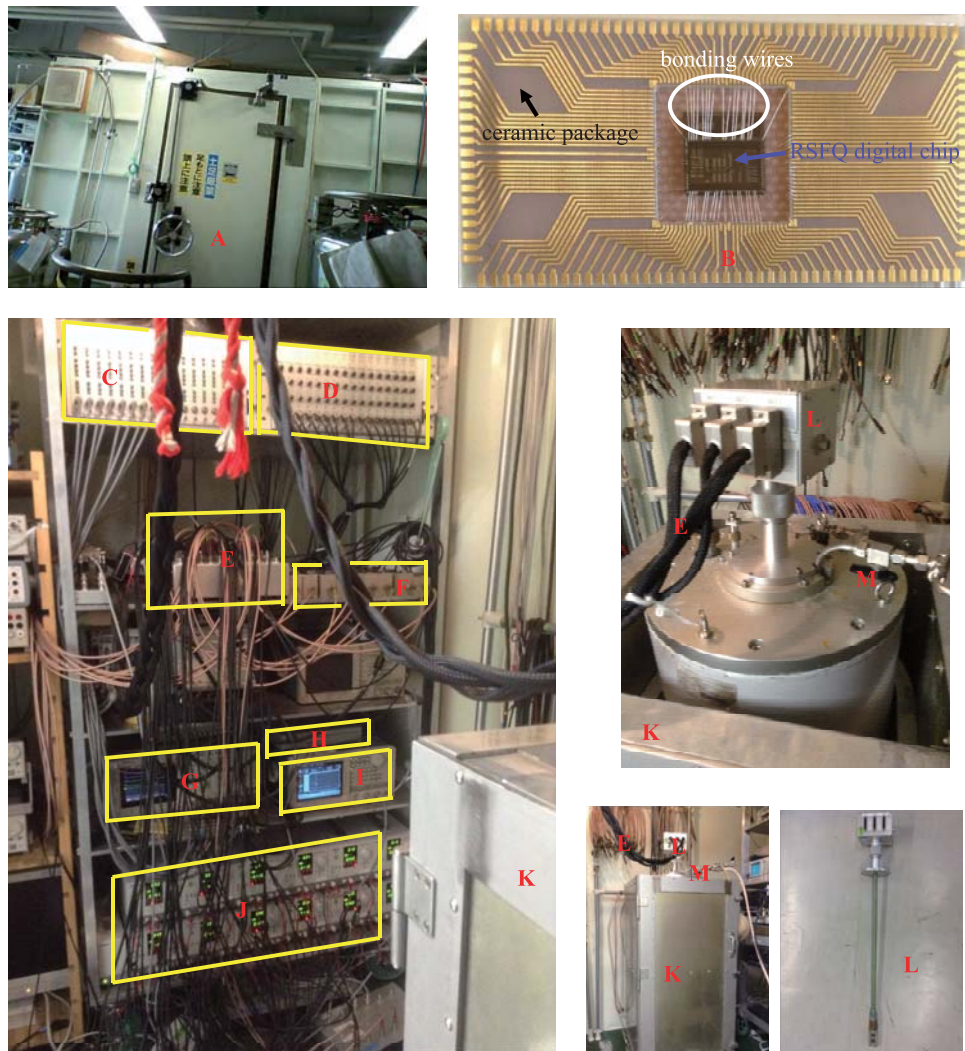
Figure 2.18. Equipment used for testing RSFQ digital chips.
