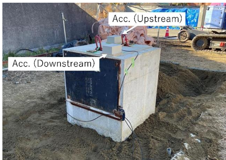
Figure 2.2 Photo at intact step with locations in accelerometers.
