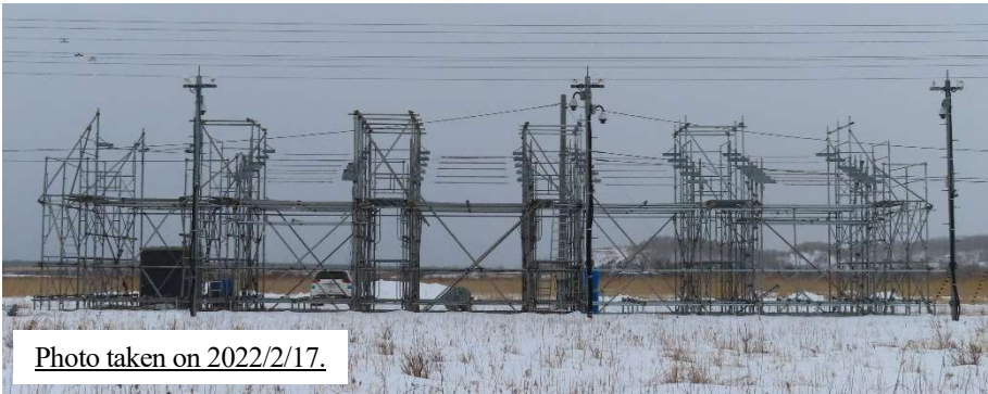
(a) Simplified observation instruments for snow accretion on conductors on the ground ( h = 4\text{ m} )
