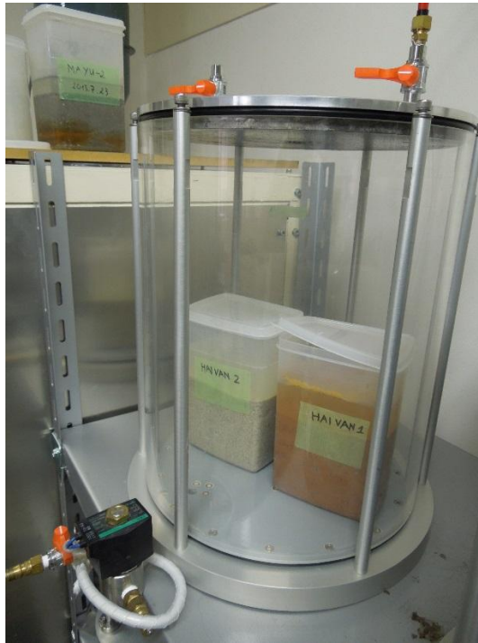
Fig. 2.8 Samples were fully saturated by vacuum tank
