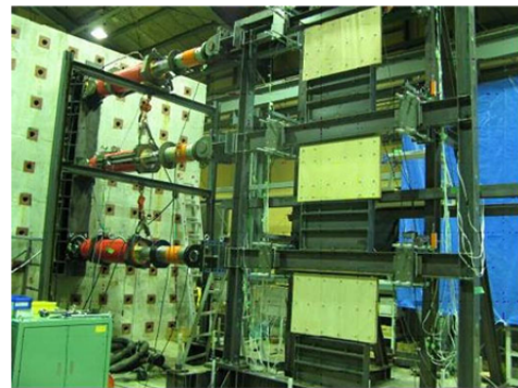
Figure 7. A steel wall with vertical slits is used as a hysteretic damper. Although the vertical slits change the mode of deformation from overall shear deformation to a series of flexural deformations and make the wall more energy dissipative, out-of-plane buckling yet occurs unless the wall is very thick. To delay such buckling even for thin walls, we enclose the wall by wood panel from both sides (top). The bottom picture shows a demonstration test of a three story planar frame in which such walls are installed. The walls are indeed energy dissipative.
