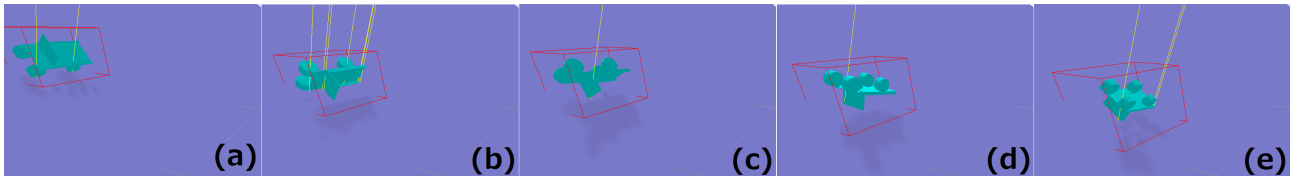
Figure 3.9: Continuous overturning behaviour in Bullet of small FWC model (TOPS height: 152 mm).
