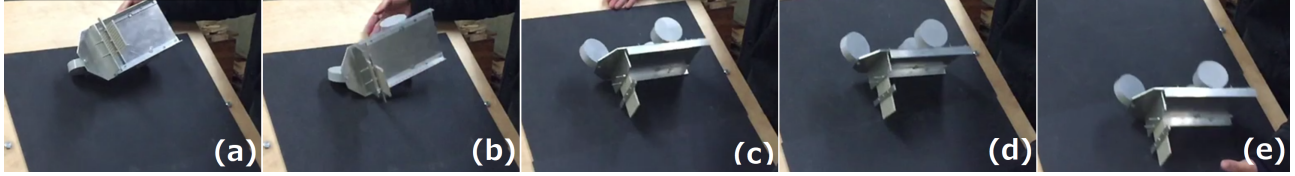
Figure 3.8: Non-continuous overturning behaviour in experiment for small TWC model (TOPS height 142 mm).
