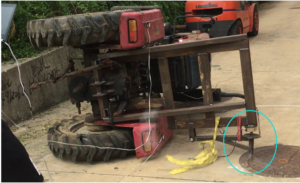
Figure 7.1: Example of overturning experiment with a designed ROPS with force sensor.
