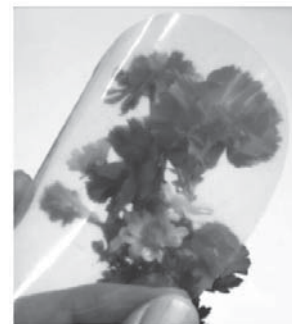
Figure 1. Wood pulp-based optically transparent nanocomposite.
