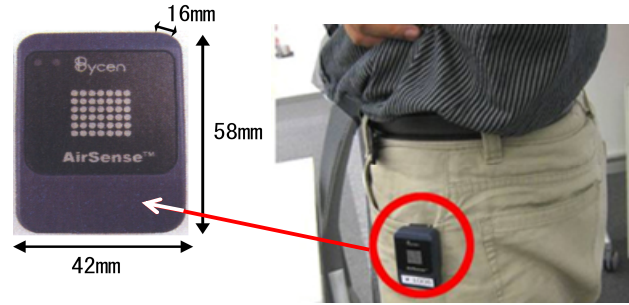
Figure 2-2 Specifications of the acceleration sensor
