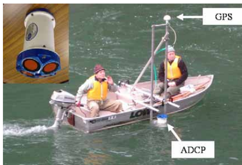
(a) Ship-mounted ADCP set-up in the field.
