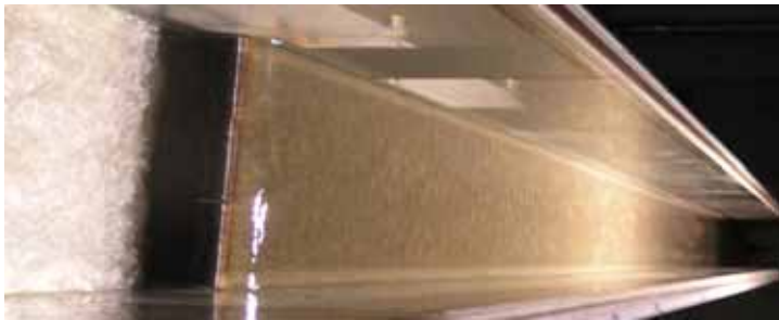
(b) Formation of experimental bed configuration (left) and flow in the vicinity of the weir model (right, 50cm x 11.5cm x 2.0cm).
