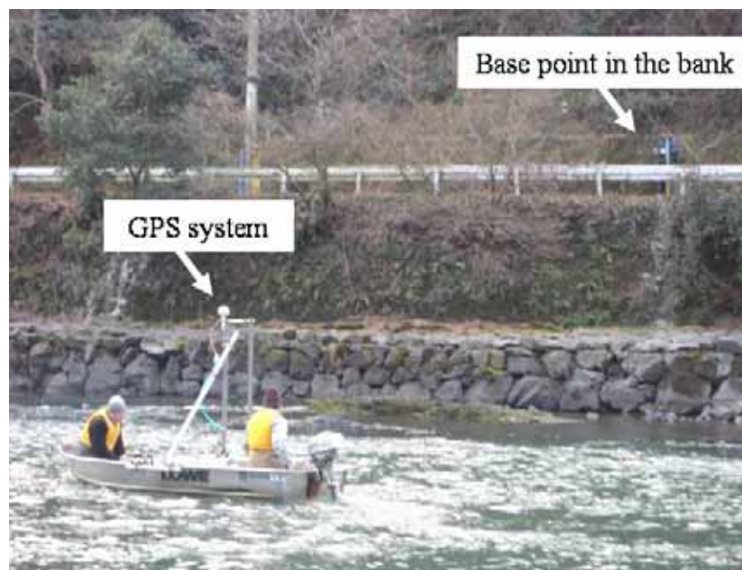
(b) Bed elevation and flow velocity measurement by ship-mounted ADCP. The location by GPS system were calibrated using the data of base point in the bank
