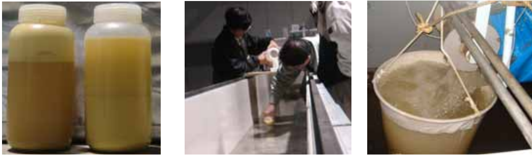
(e) Preparation of two types of pollen (left), release of the pollens at upper of the flume (middle) and collection of transported pollens after deposition to the experimental bed (right)
