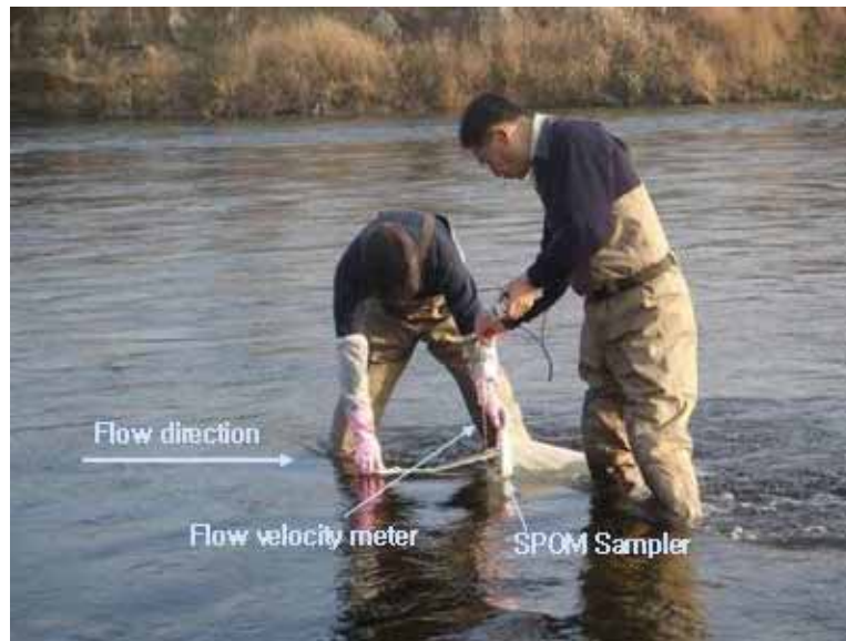
Photo 4-1 SPOM sampling using POM net in running waters in the Uji River. At the same time, flow velocity in front of net mouth and the duration time were measured for quantification of SPOM concentration.
