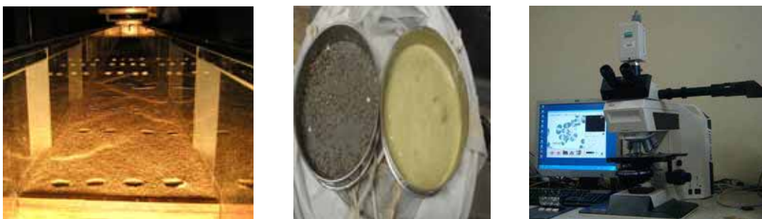
(f) Spot sampling of the deposited pollens (left) and separation of the pollens from bed materials by wet sieving technique (middle) and identification and quantitative analysis of each sample using a microscope (right)
