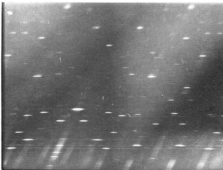
Fig. 12. (C) Weissenberg photograph of the hornblende about c-axis, heated at 1020°C for 2 hours. (zero level)
