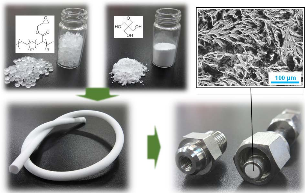
Figure 4-2. Protein A immobilized spongy monolith (ProA-SpM). Physical appearances of Pro-SpM including primary materials, a molded item, and a packed column.
