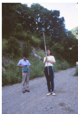
Photo 1. Profile survey of the geomagnetic total intensity across the Atotsugawa fault.
