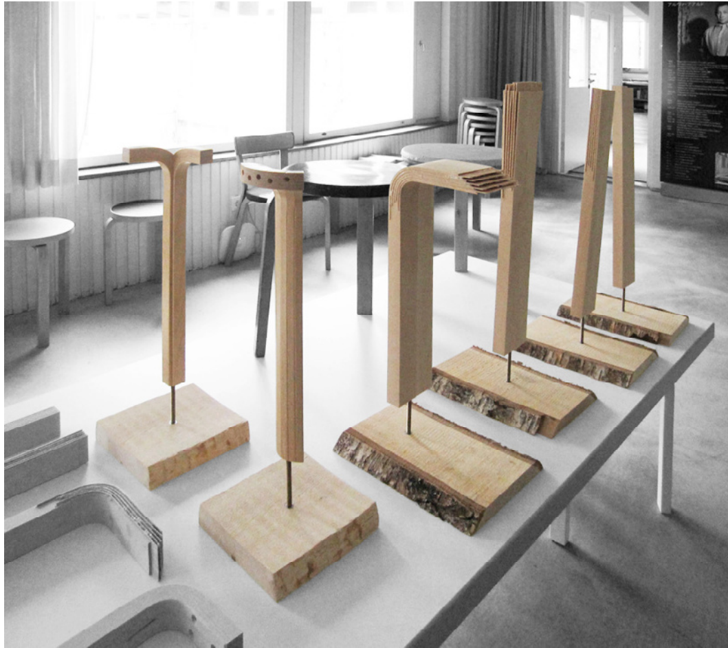
Figure 4.10. Exhibition models in the Alvar Aalto Studio showing the Y-Leg (left), X-Leg (centre), and four intermediate manufacturing stages of the basic L-Leg (right). Photograph by author.
