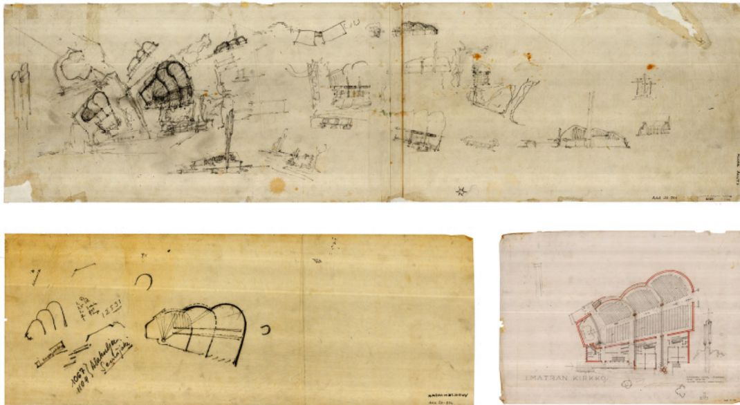
Figure 3.5. (a, top) Aalto's sketches of the church plan with freehand arcs, (b, bottom left) pure geometrical arcs, and (c, bottom right) a staff drawing dated 22 September 1955. The Alvar Aalto Museum, Finland.
