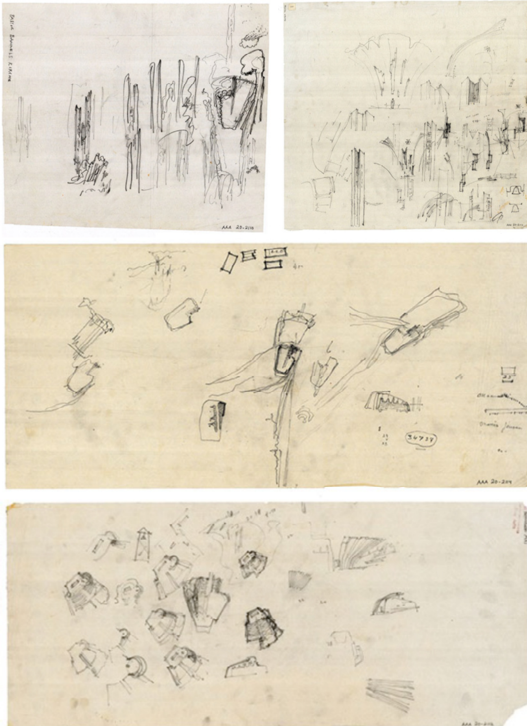
Figure 2.12. Design sketches with symmetrical and asymmetrical fan-shaped plans and bentwood sections for Wolfsburg Church. The Alvar Aalto Museum, Finland.
