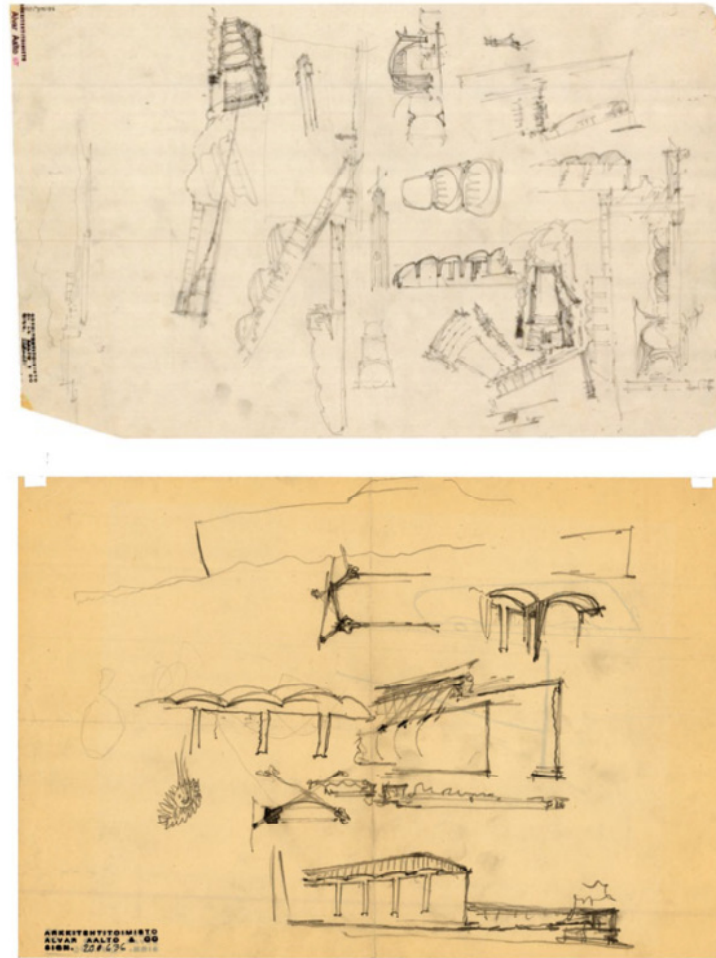
Figure 2.6. Design sketch for Seinäjoki Church showing a single trapezoidal form with repetition in both plan and section. The Alvar Aalto Museum, Finland.
