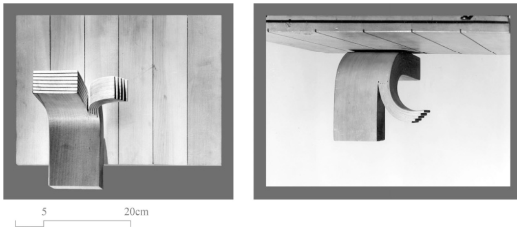
Figure 4.8. Bentwood relief from 1936 for bending in two directions, as seen from the front and above, respectively. The Alvar Aalto Museum, Finland.
