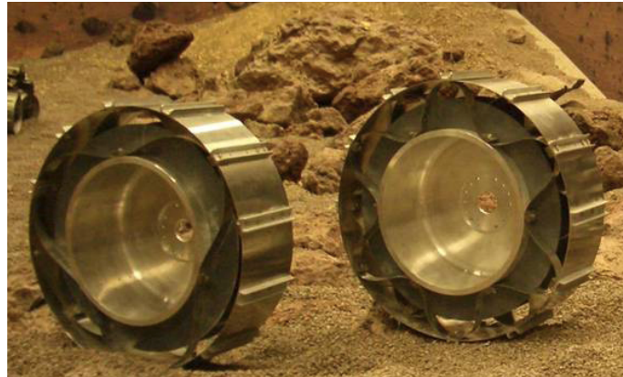
Figure 3-4: Elastic wheels in experiments (left, B3; right, B6). [9]
