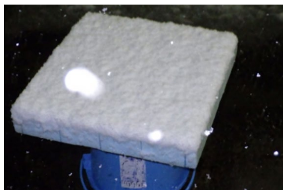
Fig. 2 Observation of the density of newly fallen snow using a snow board.
