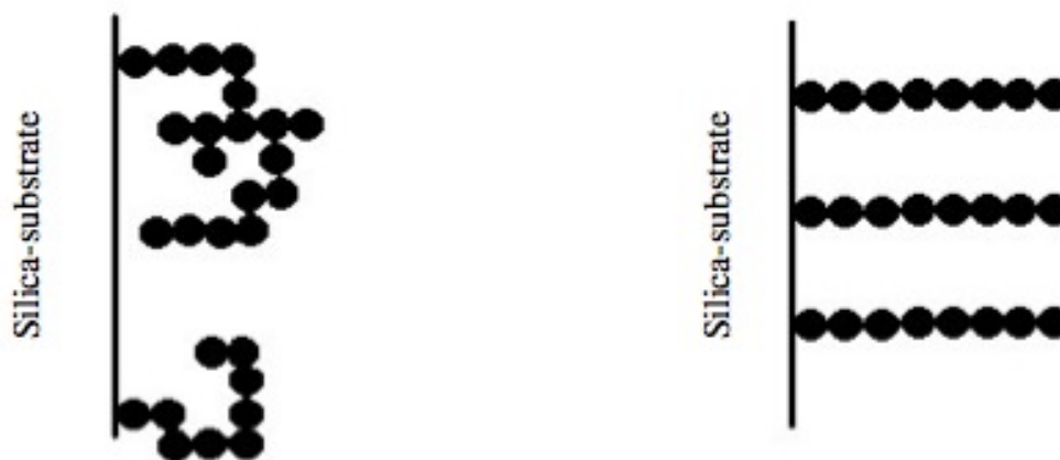
Figure 6.2 Activation of C-18 chains with organic solvent
