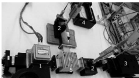
Fig.1: Photo of a 5.8 GHz PVPCM system (1: 5.8 GHz magnetron, 2: directional coupler, 3: dummy load, 4: current meter, 5: circulator, 6: spectrum analyzer.)
