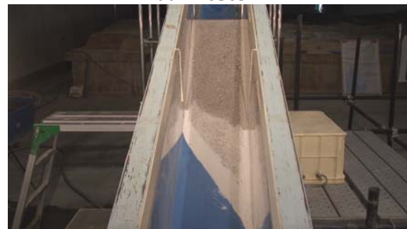
Figure 4.14 Movement of slide at different time steps - Experiment D
