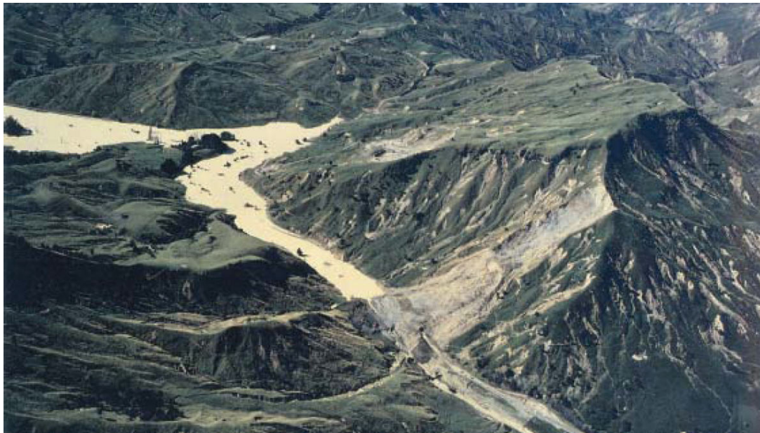
Figure 1.3 Cyclone Bola 1988 caused this large landslide in Gisborne, New Zealand, creating a lake. (Photo courtesy: www.sopac.org/tiki/tiki-download_file.php?fileId=842 , Noel Trustrum, GNS, NZ)
