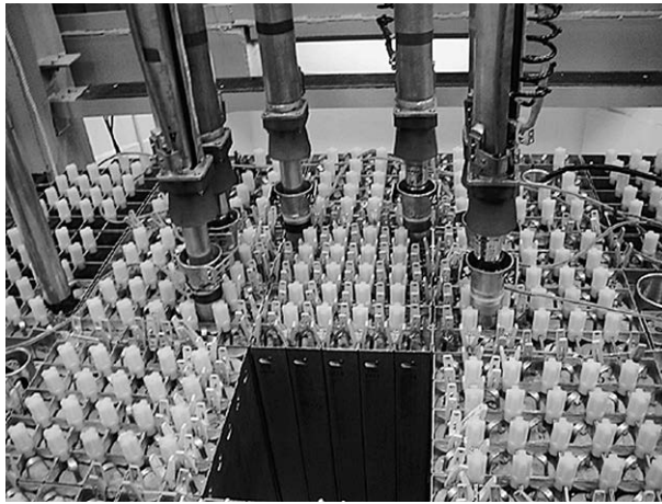
Fig. 3 Solid-moderated and -reflected core
