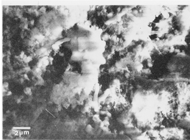
Fig. 2. High magnification of a granular cluster shown in Figure 1. The cluster consists of bacteria, apatite spherulites, crenated red blood cells and fibrin-like materials.
