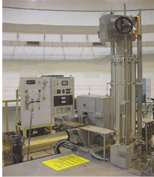
Fig.2-6 Specimen loading chamber of Materials Controlled Irradiation Facility on the top of KURR.
