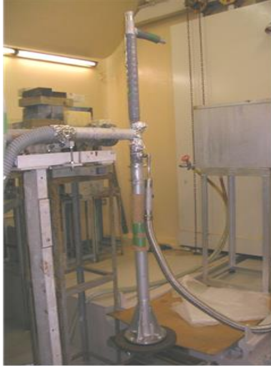
Fig.2-3 Target of electron irradiation at liquid nitrogen temperature.
