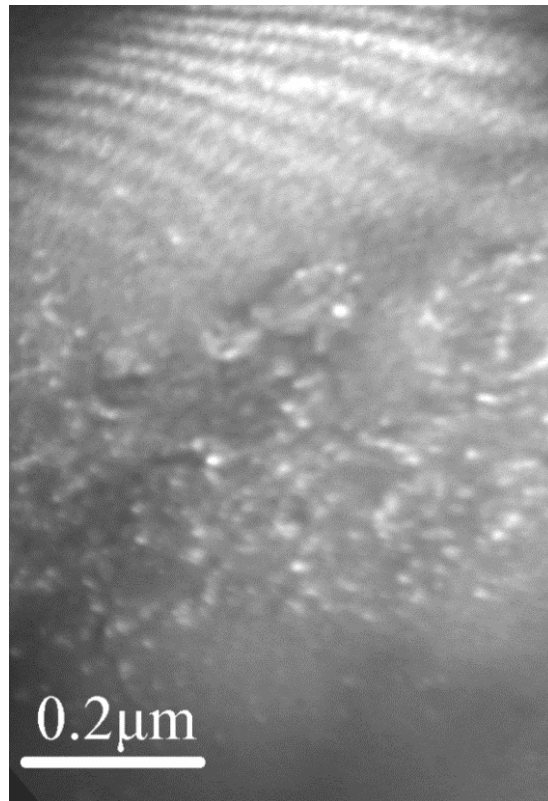
Fig.4-14 Dark-field micrograph for irradiated band area of Fe after 6 MeV Fe ion irradiation at 593 K to 22 dpa.
