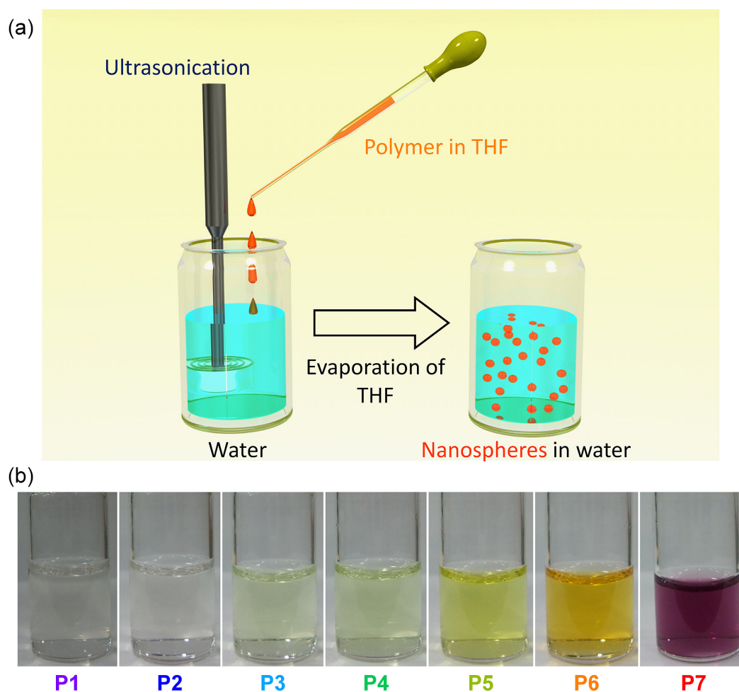
Figure 13. (a) Schematic procedure of reprecipitation method. (b) Photo images of P1–P7 nanosphere solutions in water.
