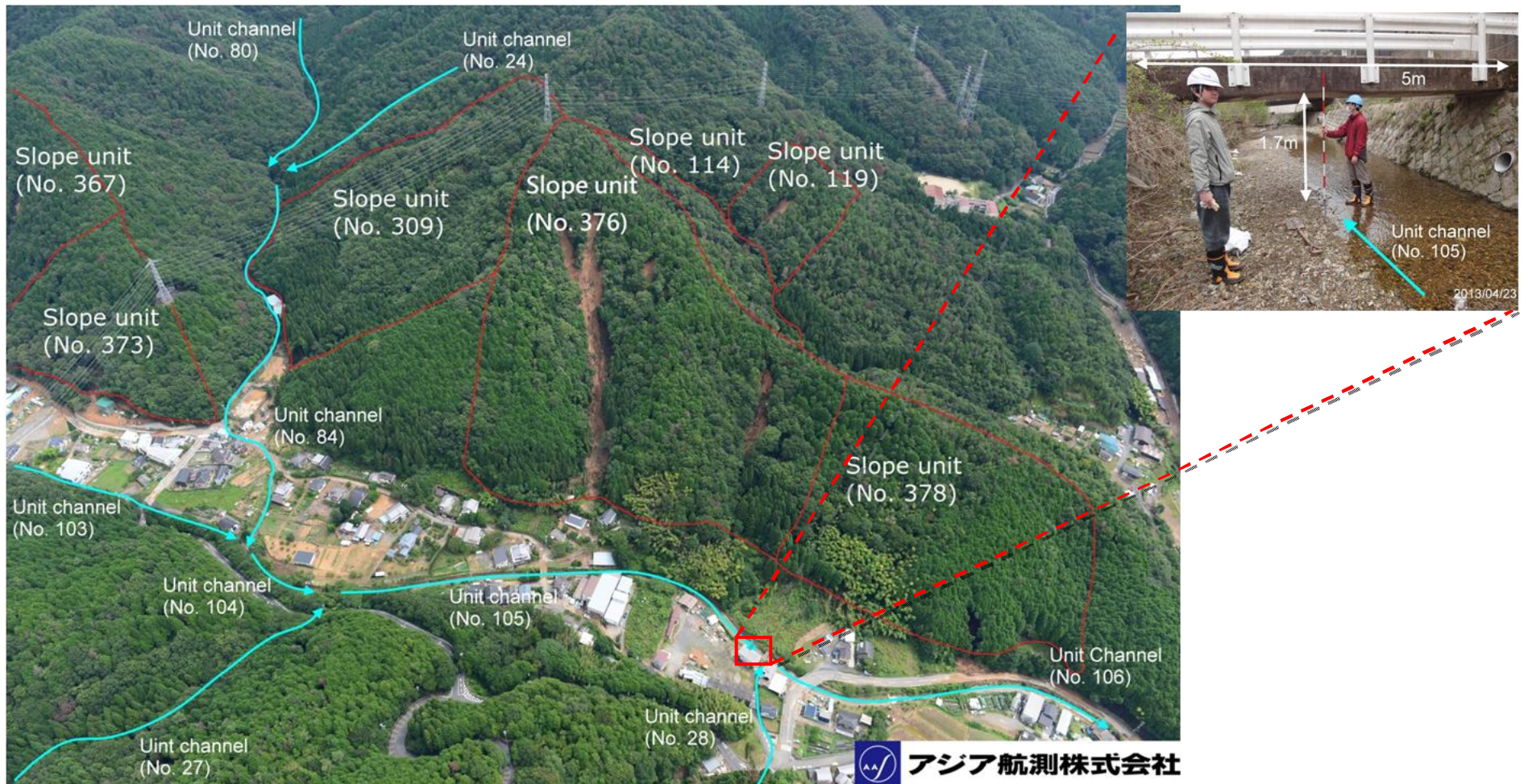
Figure 5.7 The disaster locations in Sumiyama area (2/3), and flood occurred at the unit channel of No.105 [modified from Asia air survey co., LTD , 2012]
