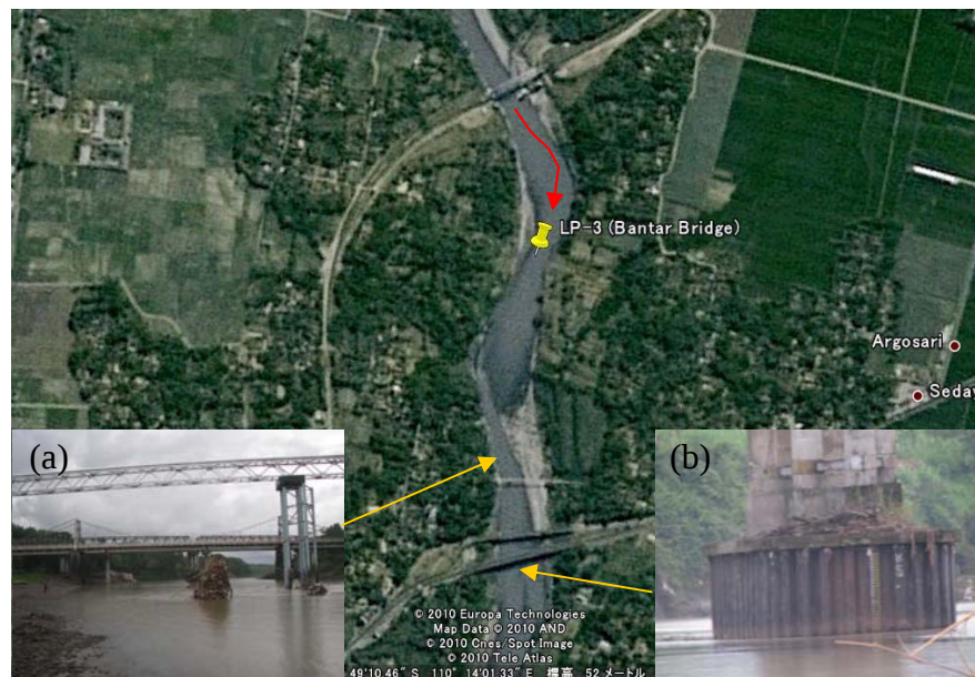
Photo 2.3 (a) The Bridges in Bantar and (b) a foundation is exposed by the riverbed degradation. The photos were taken in December 2008 (Source: Google Earth, 2010)
