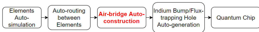
Figure 4.7: EDA process for quantum processor design, with our contribution in red. (©2024 IEEE. Reprinted with permission from [31]).
